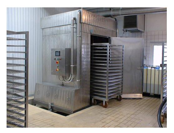
The HILLERSLEV Trolley Washing Machine is a semi automatic washing machine for standard smoke trolleys. The machine has a capacity of about 10-20 trolleys per hour.
