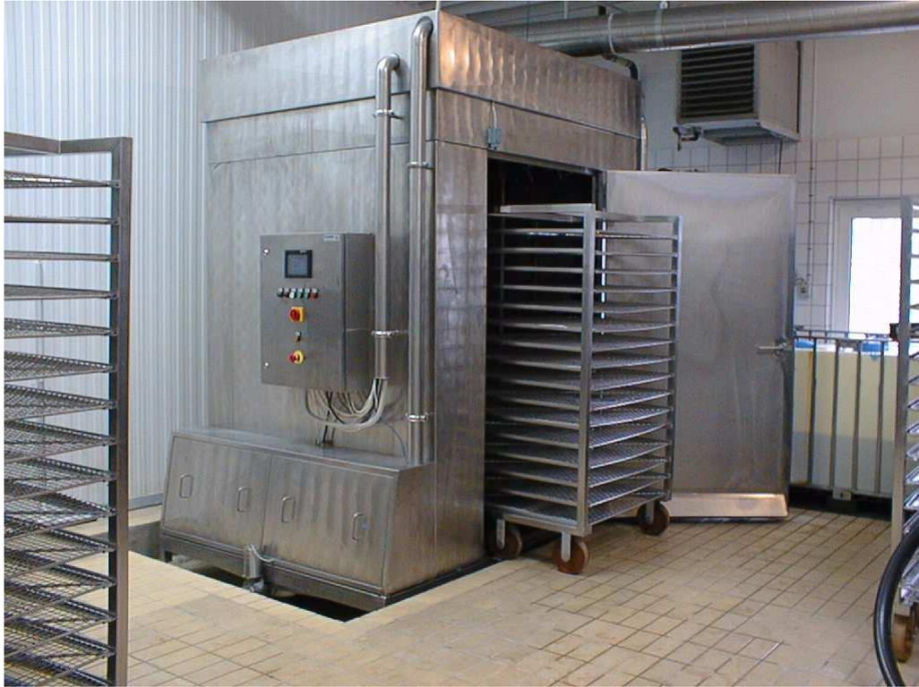
The HILLERSLEV Trolley Washing Machine is a semi automatic washing machine for standard smoke trolleys. The machine has a capacity of about 10-20 trolleys per hour.
